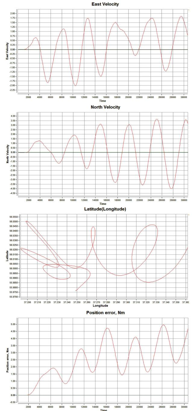
Fig. 6. IMU400 navigation performance in pure inertial mode (static), 8 hrs, no aiding, 20 min. alignment, 4 cardinal directions. East & North Velocities in m/s.
