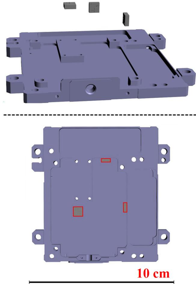
Fig. 2. Spatial displacement of 3 physical MEMS-accelerometer triads inside the IMU400. Scale bar is applicable only for the bottom drawing.
