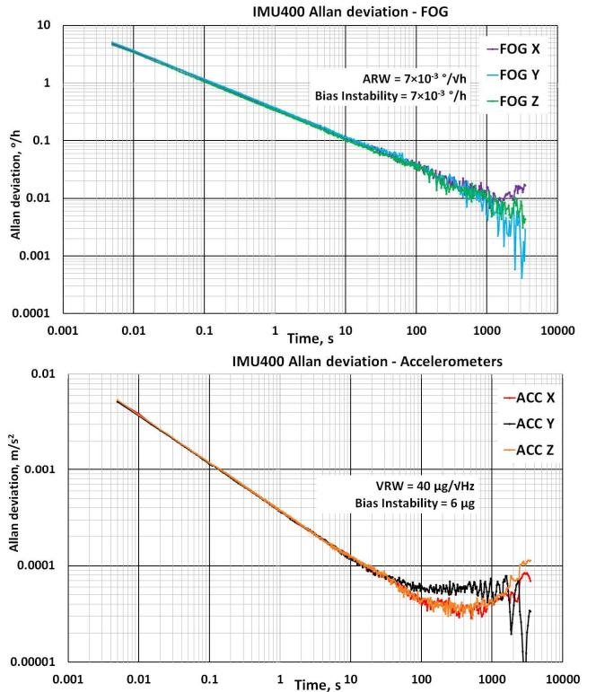
Fig. 3. IMU400 Gyroscopes & Accelerometers Allan deviation plots.
