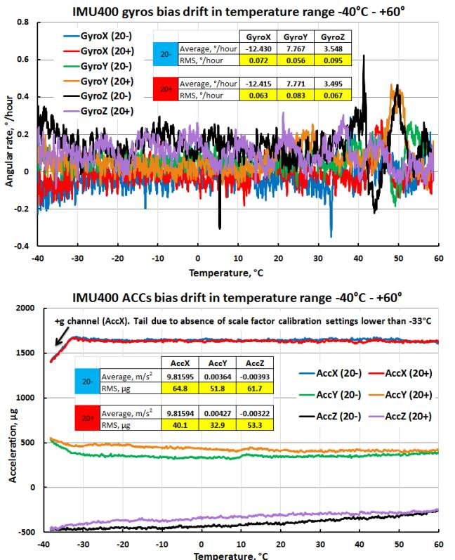
Fig. 4. IMU400 Gyroscopes & Accelerometers bias stability (drift) plots in temperature range  $-40^{\circ}\text{C} - +60^{\circ}$  with constant temperature change rate (ramp)  $+20^{\circ}\text{C}/\text{hour}$  (20+) and  $-20^{\circ}\text{C}/\text{hour}$  (20-). Absolute values are shifted.
