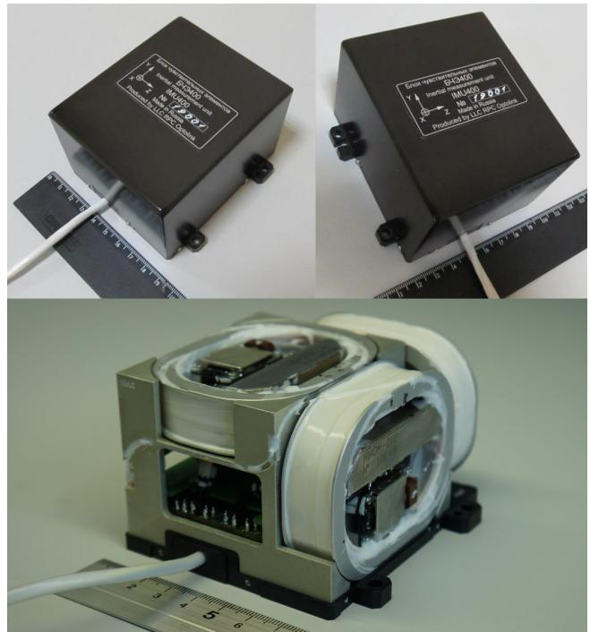
Fig. 1. IMU400 external and internal view (gyro coils).
