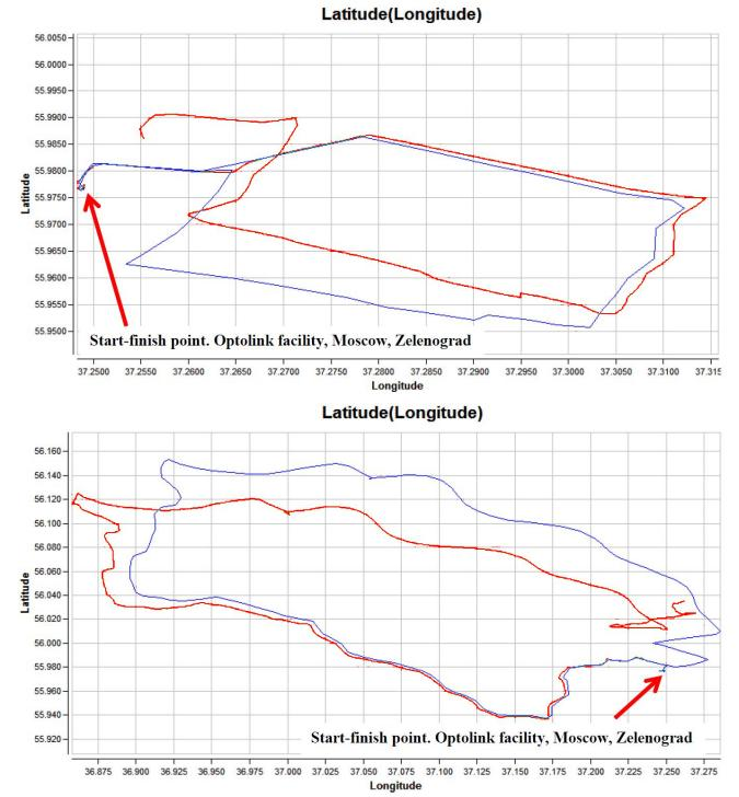
Fig. 7. IMU400 navigation performance in compensated inertial mode (ZUPT) in two data sets on tracks:  $\sim 30$  km ( $\sim 1$ km CPE error),  $\sim 110$  km ( $\sim 10$ km CPE error). Blue is GPS plot, red is IMU postprocessing track.
