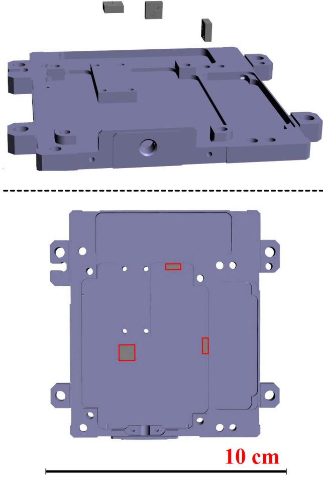
Fig. 2. Spatial displacement of 3 physical MEMS-accelerometer triads inside the IMU400. Scale bar is applicable only for the bottom drawing.
