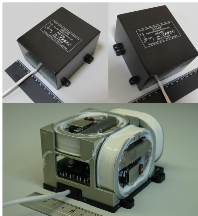
Fig. 1. IMU400 external and internal view (gyro coils).
