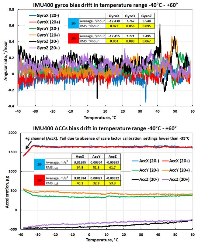
Fig. 4. IMU400 Gyroscopes & Accelerometers bias stability (drift) plots in temperature range -40°C - +60° with constant temperature change rate (ramp) +20°C/hour (20+) and -20°C/hour (20-). Absolute values are shifted.
