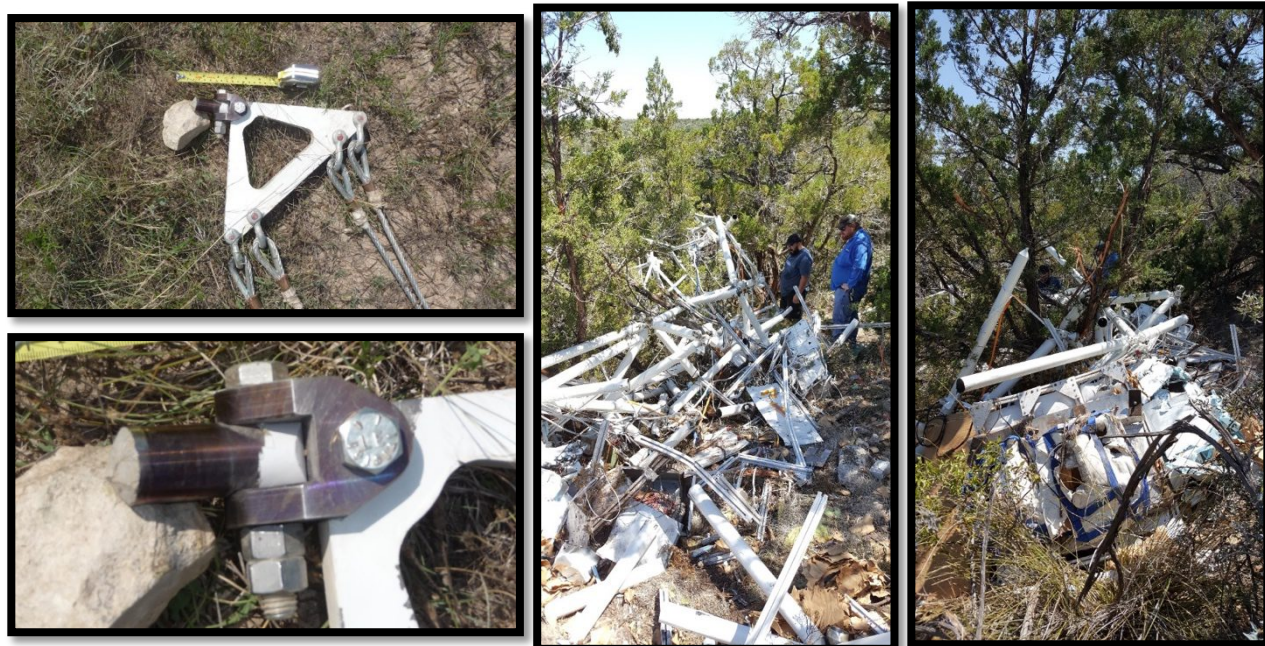
Figure 7: BETTII fell 135,000 feet in ~12 minutes: it did not survive impact. The left two pictures show the truck plate attached to the parachute, along with the rotator pin. The right two pictures show the remnants of the payload.
