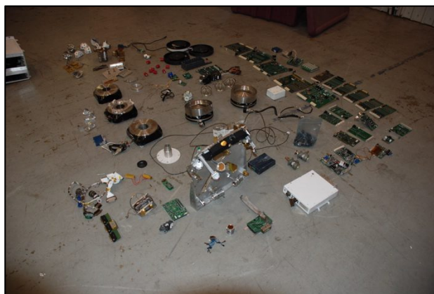
Figure 9: Triage activities allowed us to identify a number of components that were potentially reusable, including a large number of electrical components and the large mirrors.
