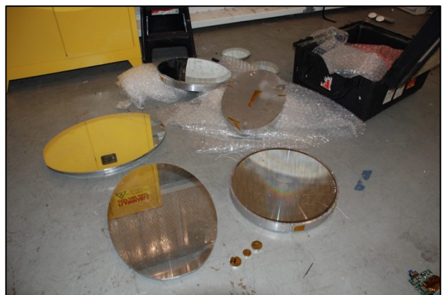
Figure 9: Triage activities allowed us to identify a number of components that were potentially reusable, including a large number of electrical components and the large mirrors.
