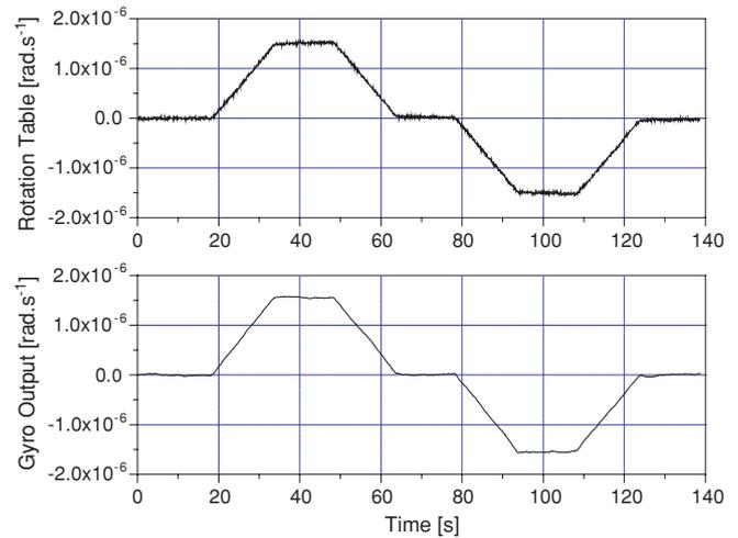
**Figure 1.** Commanded velocity profile (top) and gyroscope output (bottom).
