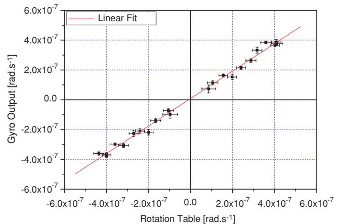
**Figure 2.** Rotation table versus gyro output for angular velocities ranging from  $0.5$  to  $2.5 \times 10^{-6}$  rad s<sup>-1</sup>.
