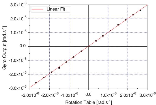
**Figure 3.** Rotation table versus gyro output for angular velocities ranging from  $1$  to  $4 \times 10^{-7}$  rad s<sup>-1</sup>.
